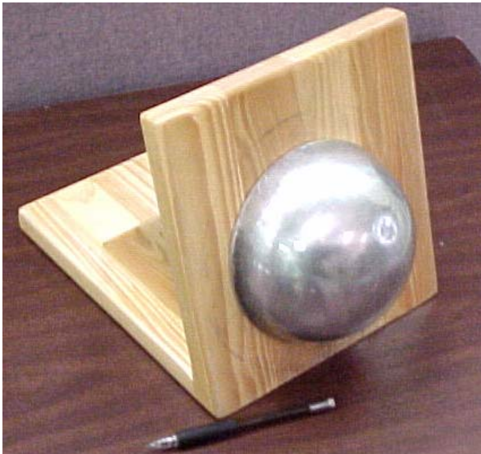
Figure 40 Simulated reflector consisting of a water filled aluminum hemisphere in testing configuration
