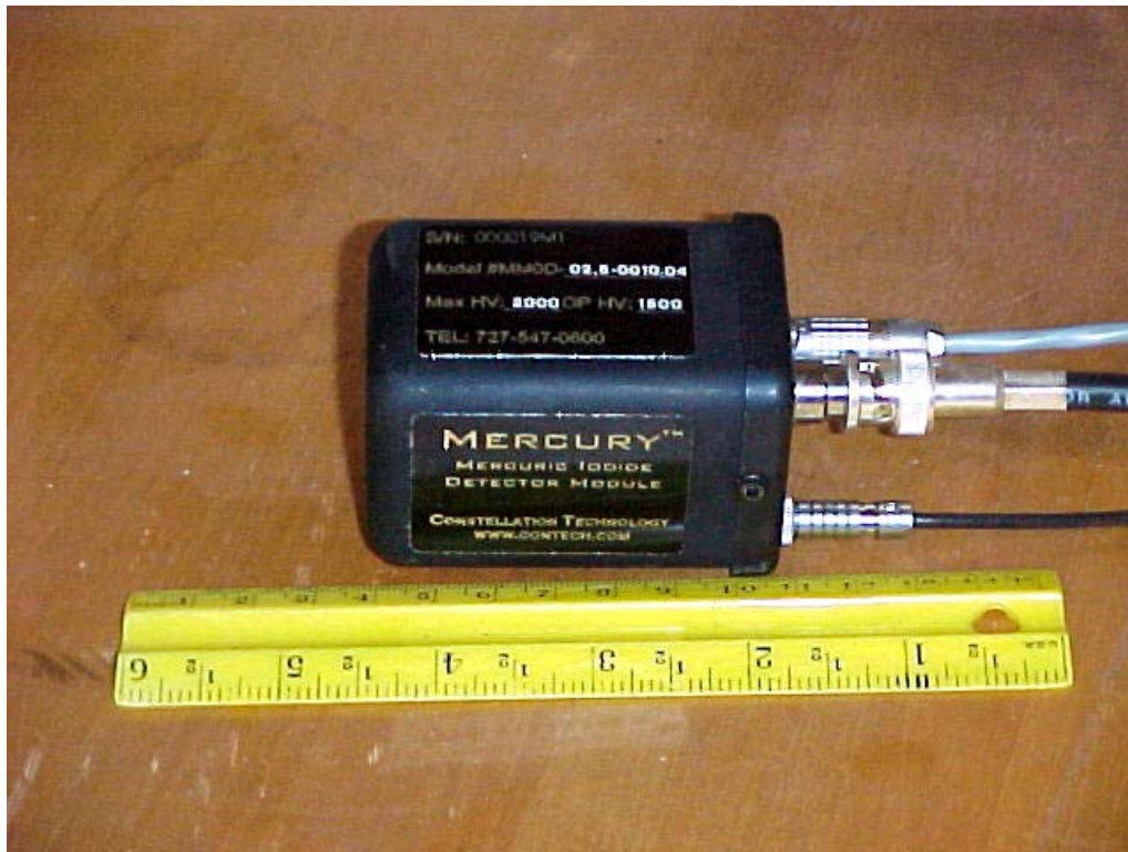
Figure 7 HgI 2 detector evaluated as part of the project
