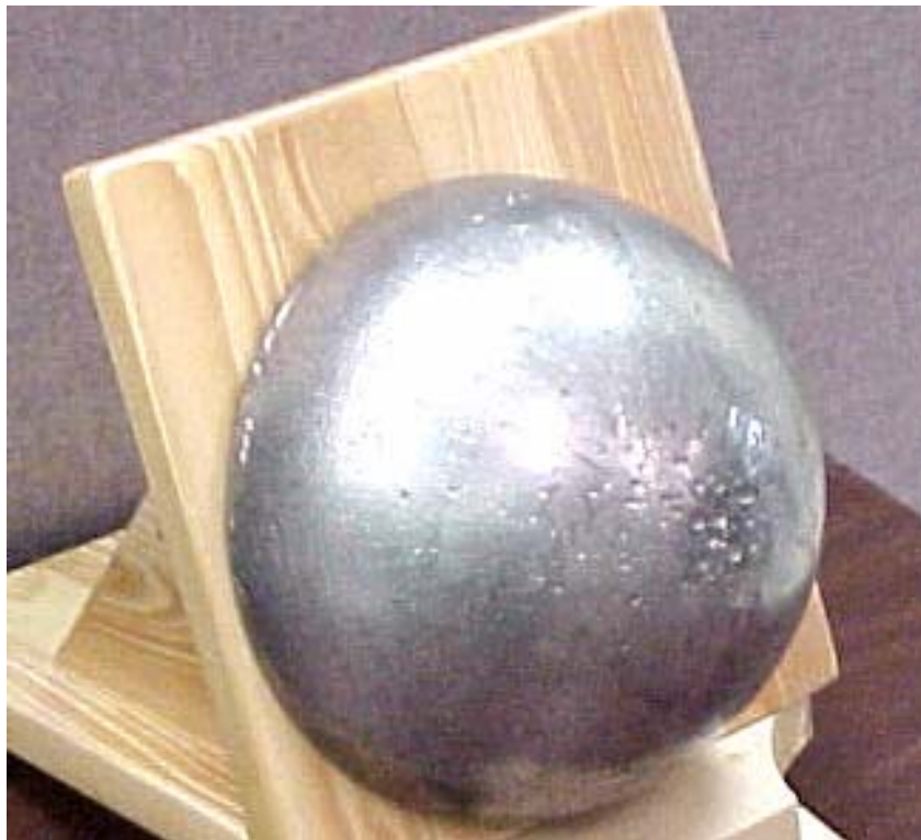
Figure 41 Simulated lead tamper in testing configuration
